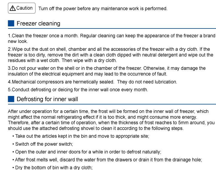
Restart the equipment after the bin is cleaned well;
